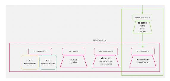
FIGURE 5.8: Firebase architecture
