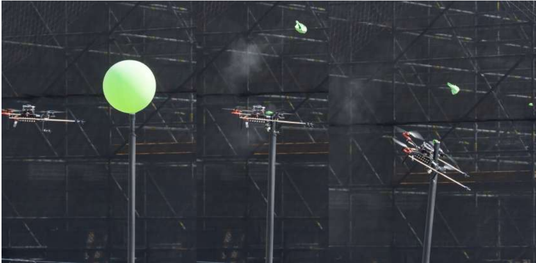
FIGURE 5.4: The UAV crashes into the metal pole because of a wrong estimated height.
