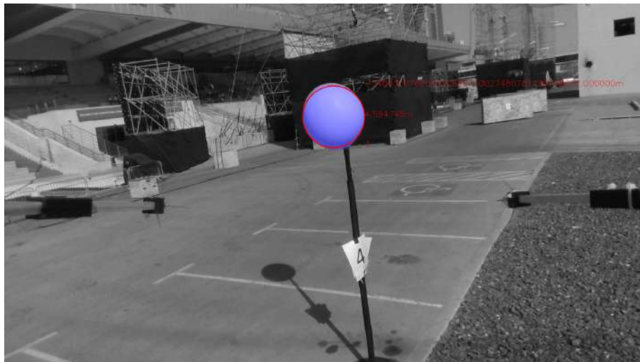
FIGURE 6.2: A debug image from onboard camera processed by Object Detect. The tracked object is highlighted by red circle.
