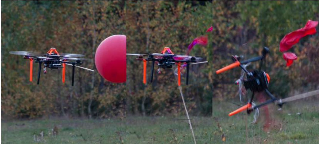
FIGURE 2.2: Drone is falling due to the balloon shred parts got stuck in the motor.
