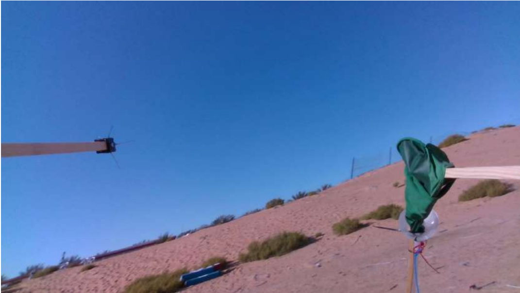
FIGURE 2.4: A photo from the drone onboard camera, when the balloon got entangled around the pole with needles.
