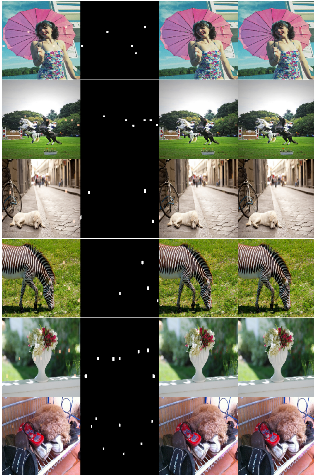
FIGURE 4.3: Bright Spots Removal with global loss function. From left to right: input image, bright spots mask, prediction, ground-truth. The mask is provided for visualization purpose only and is not used for training in this setup. The last row shows example of the input without any reflection, confirming that the model is able to detect and not damage the background layer. Zoom in for a better view.
