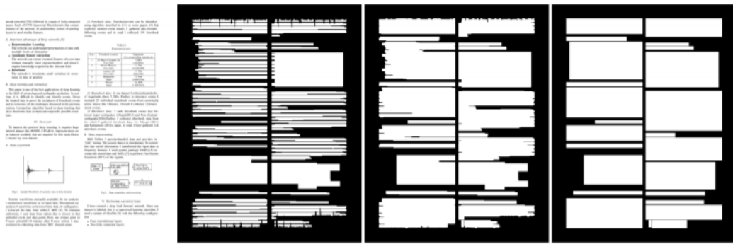
FIGURE 3.2: The process of segmenting a page into blocks of content. a) Converted to grayscale mode. b) Result image after applying RLSA (Wong, Casey, and Wahl, 1982). c) Result image after applying twice dilation by a 3 \times 3 mask. d) Resulting blocks of content. Source: Augusto Borges Oliveira and Palhares Viana, 2017
