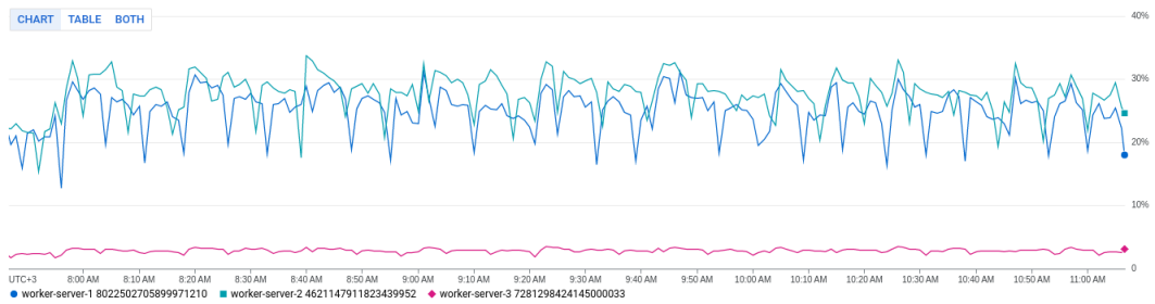
FIGURE A.13: CPU utilization chart during small request complexity test using rr algorithm
