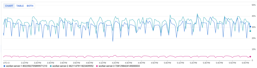
FIGURE A.9: CPU utilization chart during small request complexity test using dwrr algorithm
