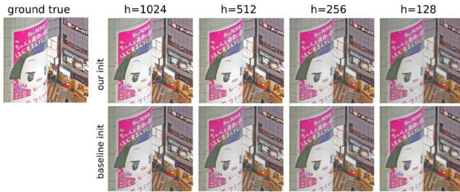
FIGURE 3.3: SIREN image representation benchmark. Models with hidden sizes of 1024 and 512 fit the image almost perfectly. Artifacts in smaller networks differ between initialization. While the networks with baseline init produce blurry results, our initialization leads to white noise artifacts.
