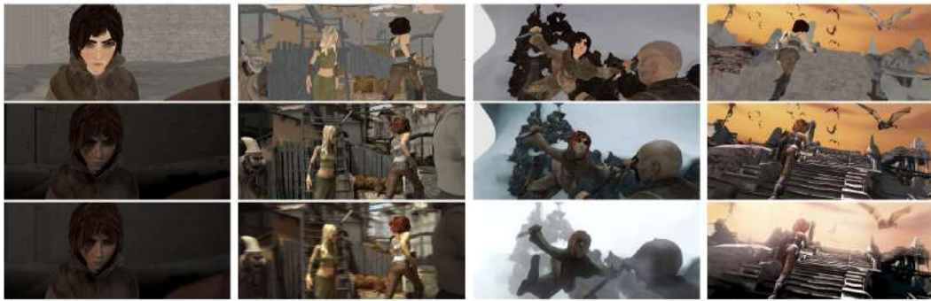
FIGURE 5.3: By row from the top: Albedo Pass (flat, unshaded), Clean Pass (smooth shading, reflections), Final Pass (rendered with large number of effects) (the image from [Butler et al., 2012]).
