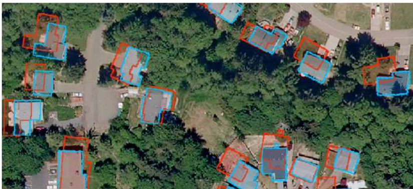
FIGURE 2.4: Results from Zorzi, Bittner, and Fraundorfer, 2020. MapRepair result. Misaligned annotations in red, corrected map in cyan.
