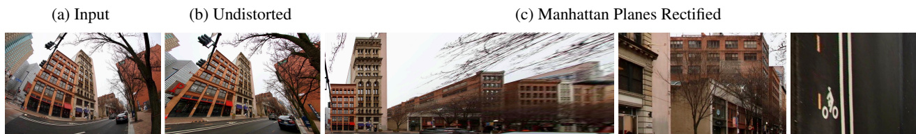
Figure 1: (a) Input is an image. (b) Lens distortion corrected, and (c) Scene planes rectified. The method is fully automatic.
