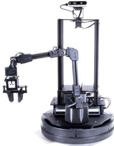
FIGURE 3.1: LoCoBot (an open source low cost robot).
