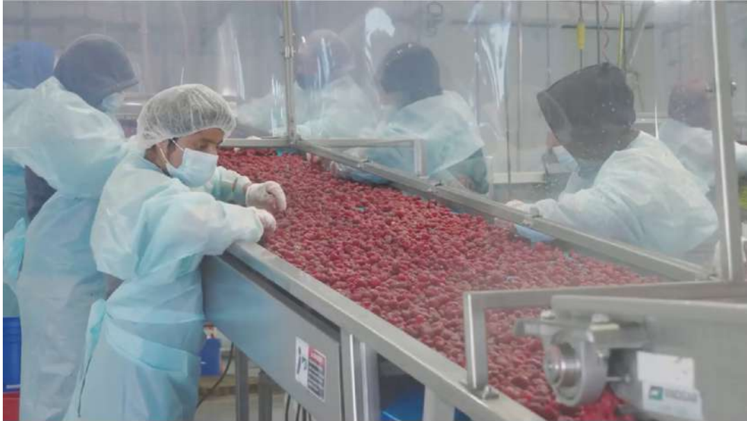
FIGURE 4.2: Manual sorting and final quality inspection of raspberries in a freezing tunnel at a temperature of -2 Celsius [WRRC, 2021]
