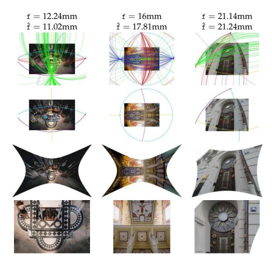
FIGURE 5.6: *Real Data Experiments: Challenging Images.* The proposed solvers were tested on challenging images taken by various cameras with different fields-of-view and distortions. Presented are examples of estimated focal length (top title), visual outputs: vanishing point labeling of arcs and region correspondences (first row) and vanishing line labeling of regions (second row); radially undistorted (third row) and metric-rectified images (bottom row).
