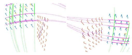
FIGURE 5.1: *Examples of Synthetic Scenes Used for Evaluation*. Illustrated are imaged two orthogonal scene planes each containing affine-covariant features arranged in a lattice (colored blue and red). The dominant scene plane (blue) also contains sets of parallel lines corresponding to orthogonal directions (colored green and magenta). The scene planes also incorporate outliers (yellow
