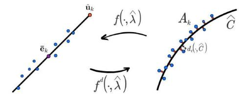
FIGURE 4.3: Arc Consistency Measure. An algorithm for computing a circular arc consistency with the model is similar to [37]. An line joining the geometric median of points and the estimated vanishing point  $\hat{\mathbf{u}}_k$  of the scene plane line direction is calculated according to (4.20), then distorted (on the right) with an estimated radial division model parameter, and the sum of orthogonal distances to a circle  $d_l(\mathbf{x}, \mathbf{C})$  is computed.
