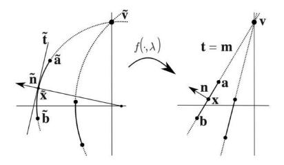
FIGURE 4.2: *Geometry of a Distorted Line.* Barreto et al. [5] showed that under the division model of lens distortion, a straight line is imaged as a circle. When undistorted, a tangent **t** to the detected circular arc is transformed such that it coincides with the original straight line [41] in the undistorted image space that passes through the vanishing point under a perspective view of a scene. The figure is adapted from [41]
