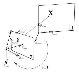
FIGURE 3.1: *Camera Viewing a Scene Plane.* Coplanar scene points  $\{X_i\}$  are assumed to be on the scene plane z = 0. The assumption implies that a homography can transform a point **X** on the scene plane in the world coordinate system to an image point **x** in the camera's image-plane coordinate system.
