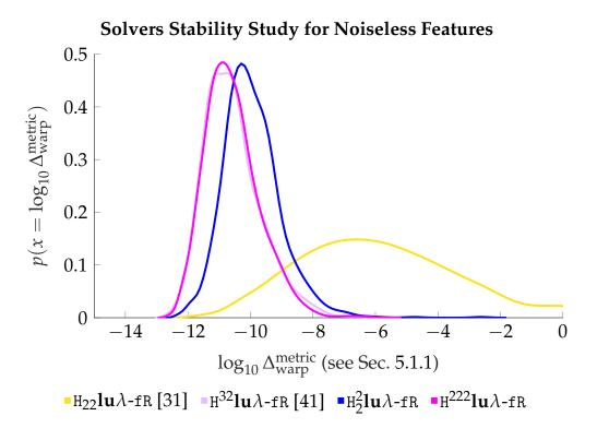
FIGURE 5.2: *Numerical Stability.* For the synthetic experiments, the normalized division model parameter is set to -4, focal length and camera pose are generated randomly within realistic bounds such that the synthetic camera is close to GoPro Hero 4. The RMS metric warp error is reported, which accounts for all the estimated calibration parameters  $\lambda$ , *f* and *R*. The proposed solvers are stable.
