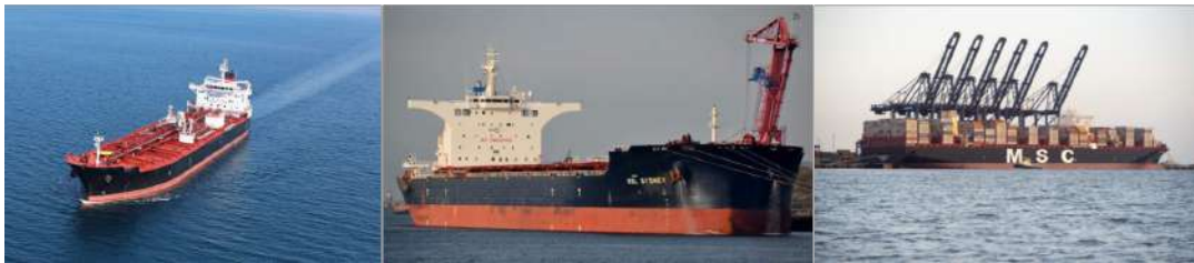
FIGURE 2.1: Different types of vessels: left - tanker; central - bulk carrier; right - container ship Source: Different kind of vessels
